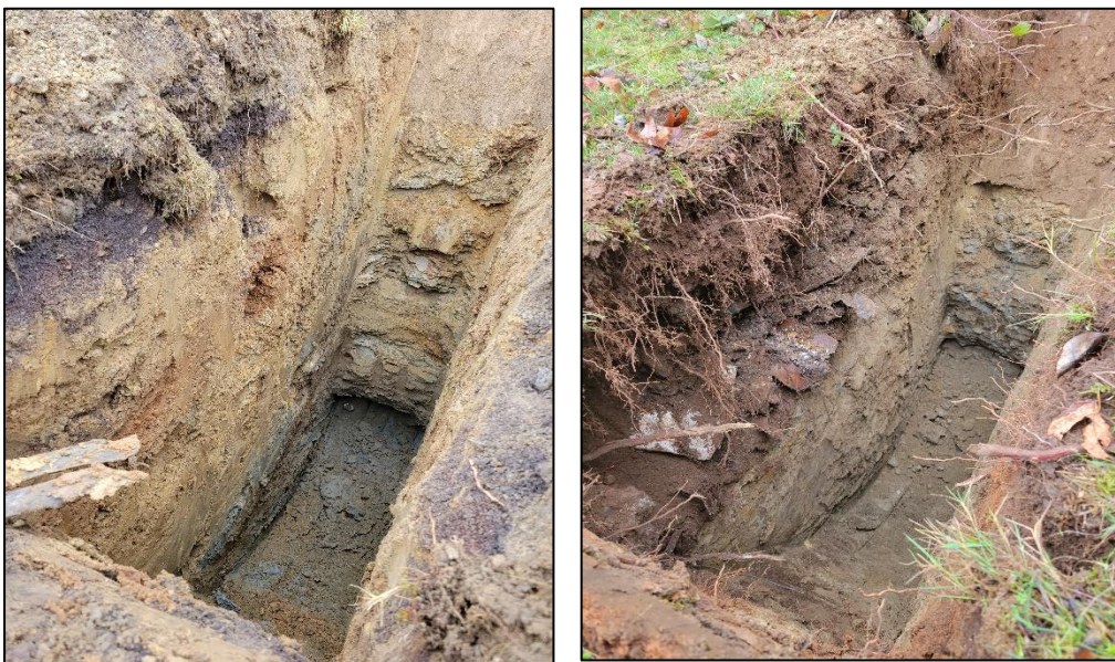
Image 3 (left) and Image 4 (right) – General subsurface conditions observed at the subject property. Image 3 shows subsurface conditions in TP-4. Note previously placed fill soils and debris atop native soils at depth in TP-5. Photos taken January 27 th , 2023.
